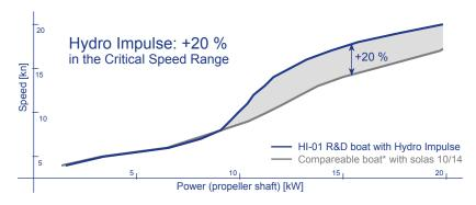
In addition to the +20% increase in efficiency in the critical speed range, the Hydro Impulse extends the range of electric boats by around 20%. Moreover, it delivers significantly enhanced acceleration from both standstill and cruising speeds, as well as improved precision and responsiveness in steering, enabling noticeably faster slalom course completion.
